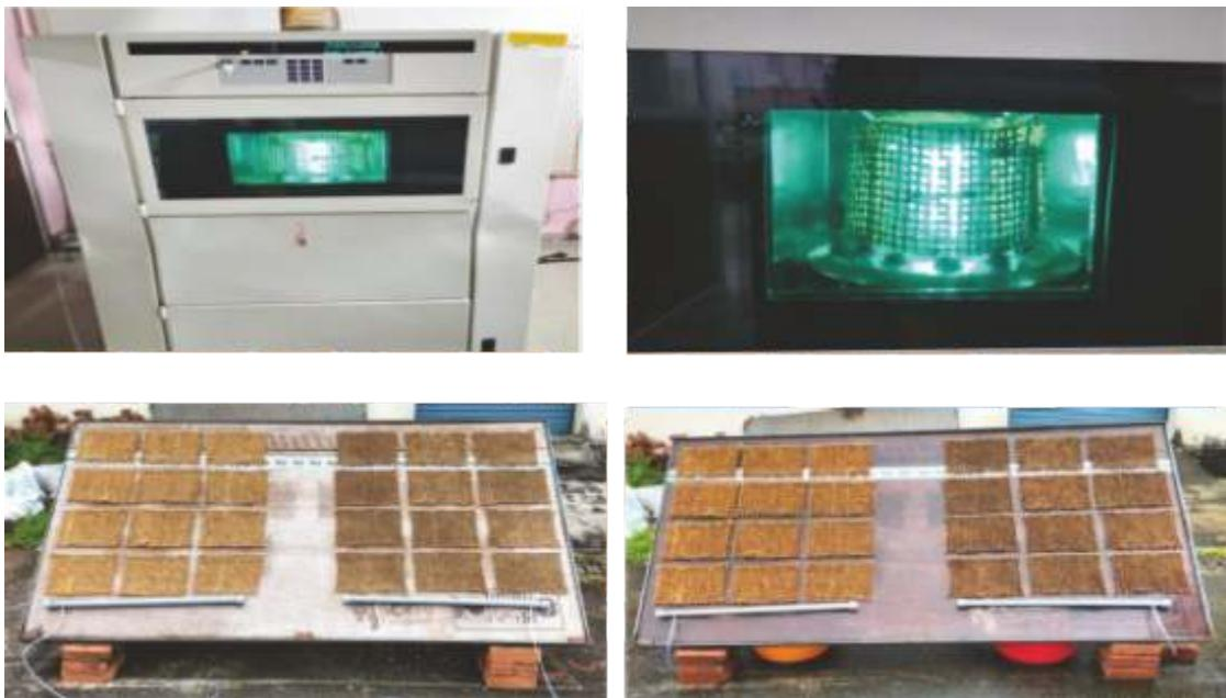
The test frames for exposure to weathering have been fabricated by the engineering department of CCRI. Arrangements have also been made to collect the leachate and evaluation of its contents.
