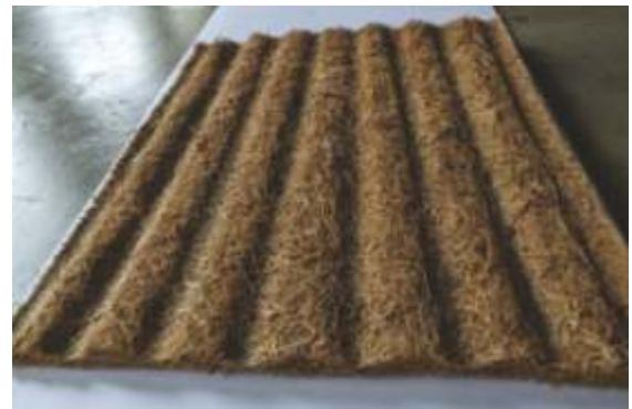
In order to provide more spongy effect without increasing the density of coir sheets, we designed it in a corrugated / projected way. This will trap air within the design providing a lighter weight experience. As the
