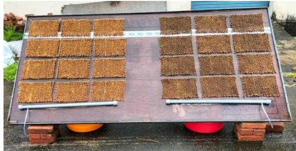
The test frames for exposure to weathering have been fabricated by the engineering department of CCRI. Arrangements have also been made to collect the leachate and evaluation of its contents.
