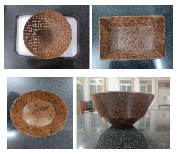
Handmade papers were prepared by existing pulp making method with the application of Tender coconut fiber / baby fiber, paper wastes and Hibiscus plant leaves in various proportions.
