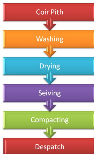
High electrical conductivity (EC) of coir pith is the major constraint in using it as growing medium. The higher level of EC in pith is rectified by washing it with good quality fresh water. Hence washing is the significant stage in the process.
