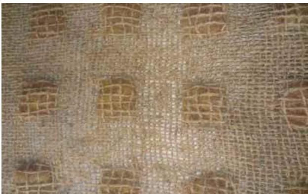
textile holds the packing material. Seed and manure can be inserted in the pockets before laying. It also avoids spreading fertile soil in the top of the mine dumping yards. The product was launched by Shri. Giriraj Singh, the Hon'ble Minister of State for MSME.
