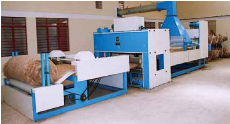
Indigenous Coir needled felt machine
