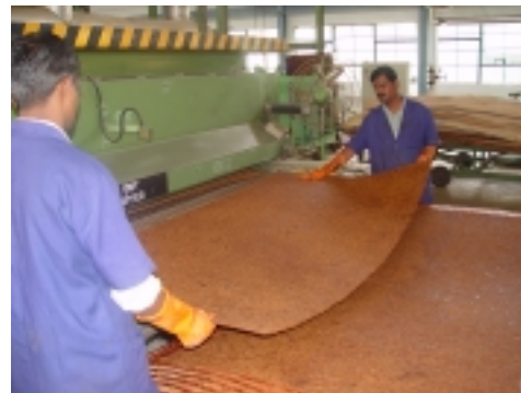
Drying of Resin Coated Coir Felt
