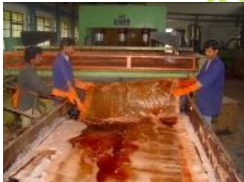
Squeezing of excess resin from Coir felt
