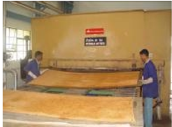
Hot Pressing of Coir Corrugated Sheet
